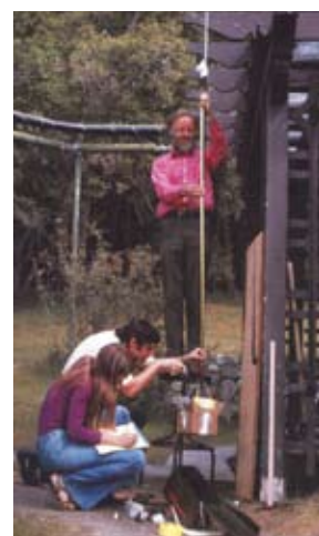
Steve measures the tensile properties of a Nereocystis luetkeana stipe with John Gosline and Mimi Koehl, circa 1975
